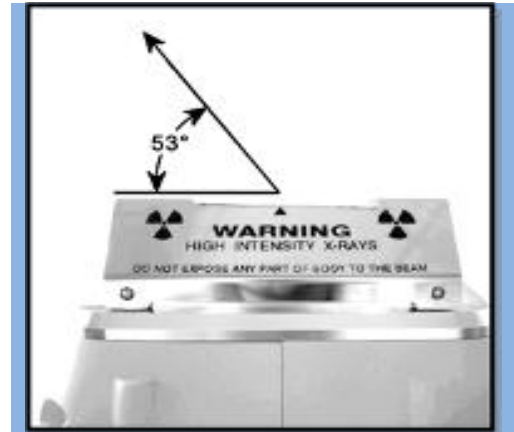
Figure 1 Emission of X-rays from the aperture
