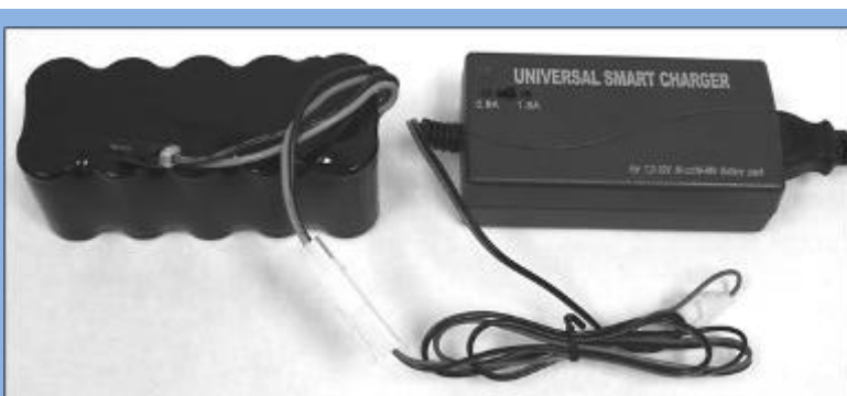
Figure 16 Charging Pump Battery
